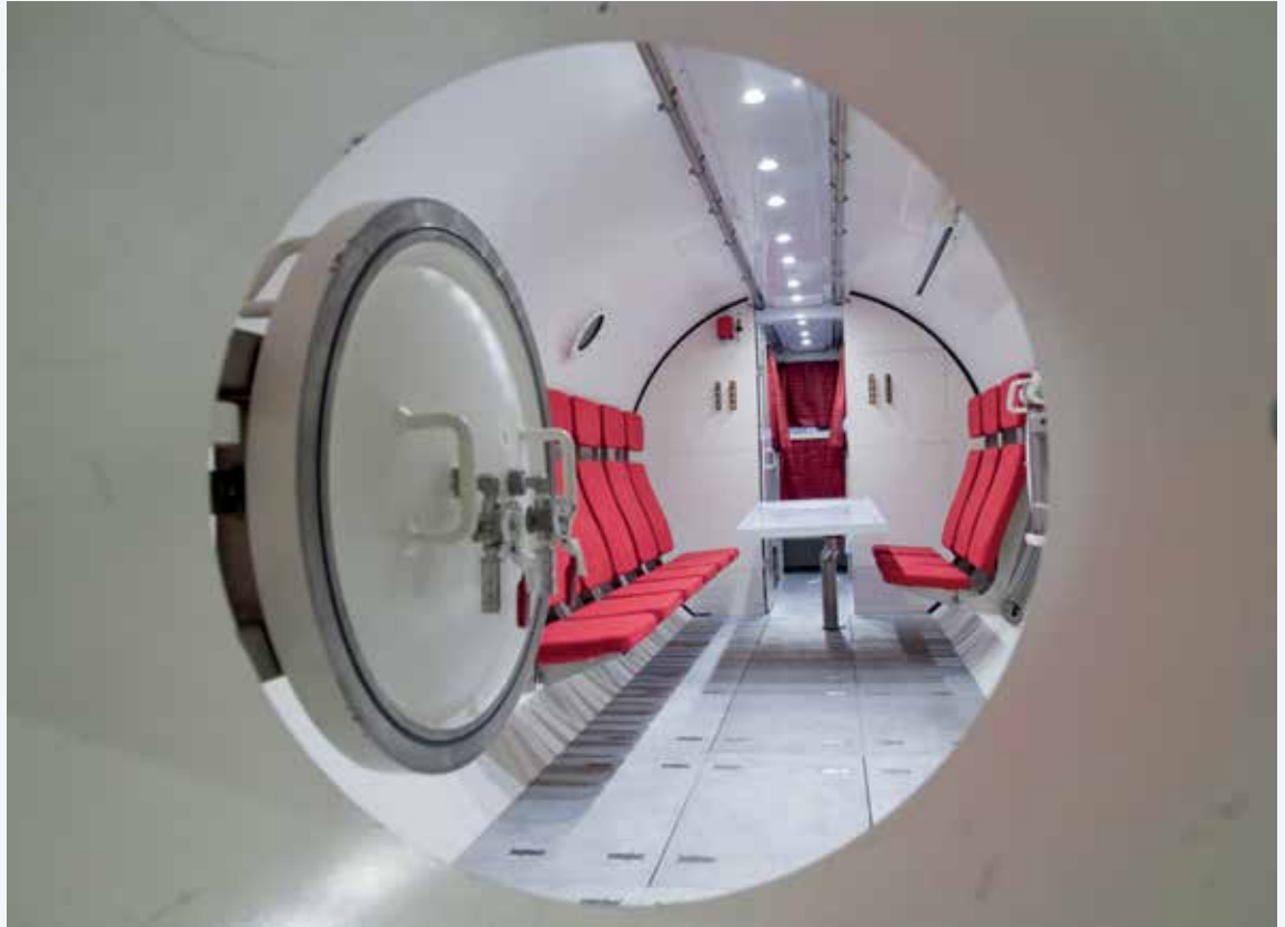
The internal chamber of a 24-man saturation diving system, one of many specialist pieces of equipment supplied to the offshore oil industry by James Fisher.
